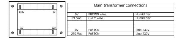
Connect power line to the transformer.
