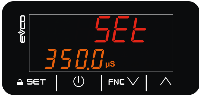
Fig. 17. First start-up - Setting the electrical conductivity
