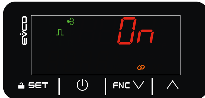
Fig. 19. Home screen with ON/OFF regulation from digital input (CFG = 0-1)
